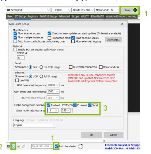
If the motor still does not connect, select every baud rate one by one in the "Baud: " dropdown menu next to the scan button. If this does not work, follow the instructions in section 4: Force updating firmware.
