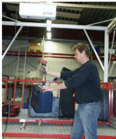
Lifter with hand-held gripper and the box containing the built-in MAC800 servo motor
