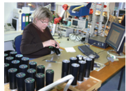
Assembly and QA of MAC140 motors
