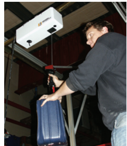
Close-up of the battery supplied gripper with buttons for controlling up and down movement of the lifter
