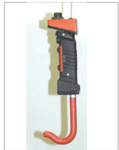
Close-up of the battery supplied gripper with buttons for controlling up and down movement of the lifter
